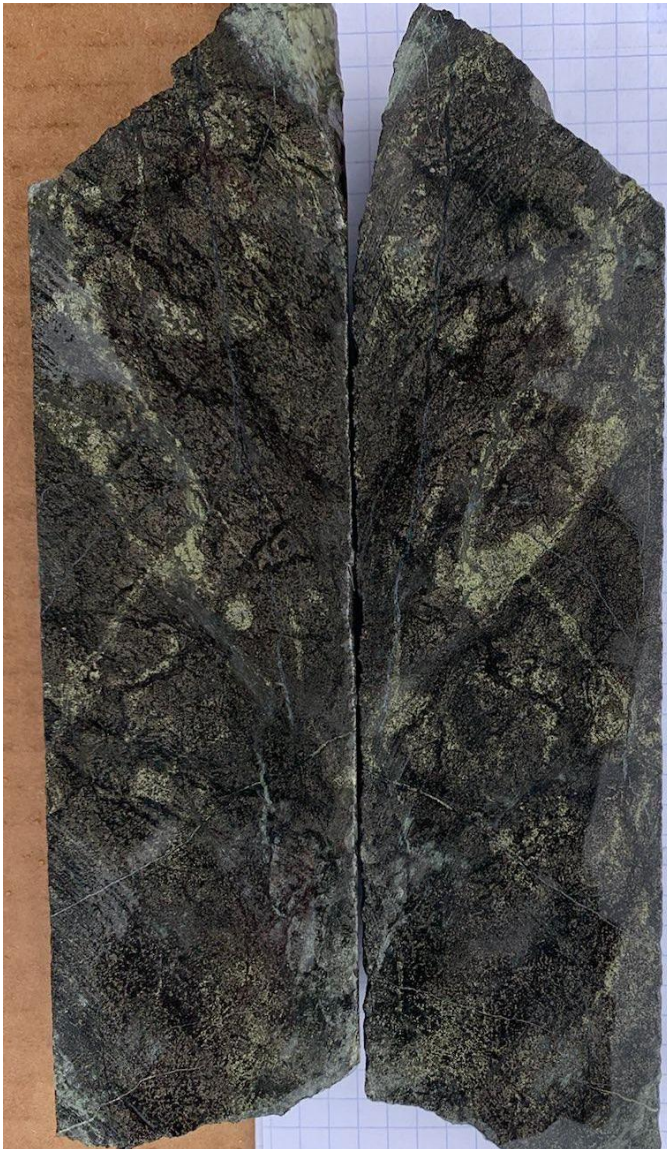
Photo 1. Drill hole TK6 at 1,042.4 m (3,420 ft) depth. Sulfide-rich magnetite breccia in 70.1 m (230 ft) core interval of the “Eureka” skarn zone
