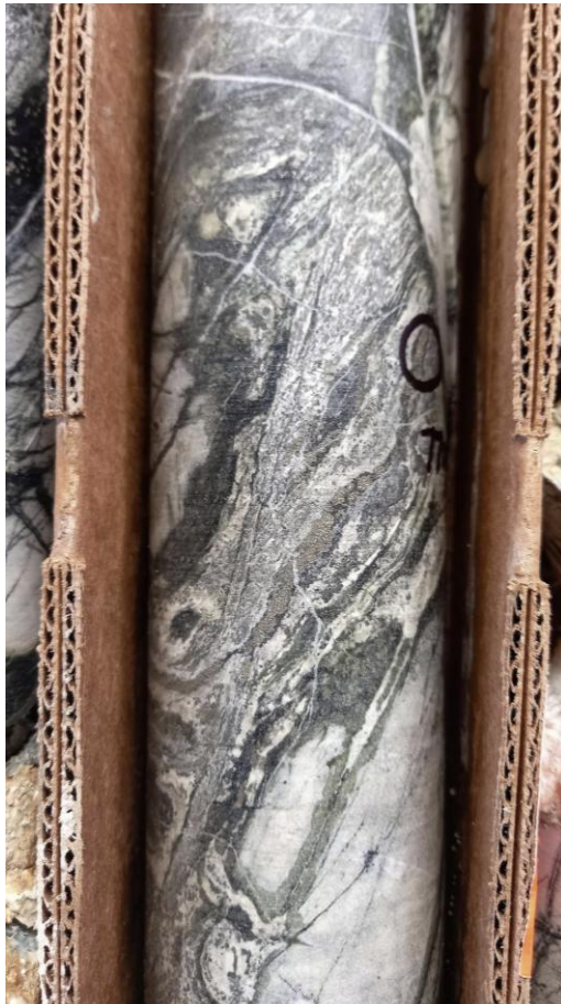
Photo 3. TK8 drill hole interval from 664.5-667.5 m (2,180 to 2,190 ft) with intense sulfide-magnetite brecciated marble skarn that assayed 1.05% Cu, 0.18 g/t Au, 0.005% Mo
