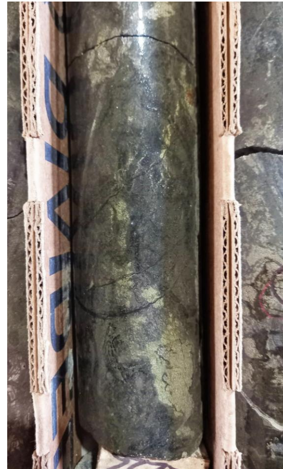
Photo 4. TK8 drill hole 10-ft (3 m) interval from 676.7-679.7 m (2,220 to 2,230 ft) detail with massive sulfide-magnetite-diopside breccia skarn that assayed 1.32% Cu, 0.29 g/t Au, 0.002% Mo
